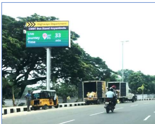
Figure 21.1: Typical Variable Message Sign Board VMS
